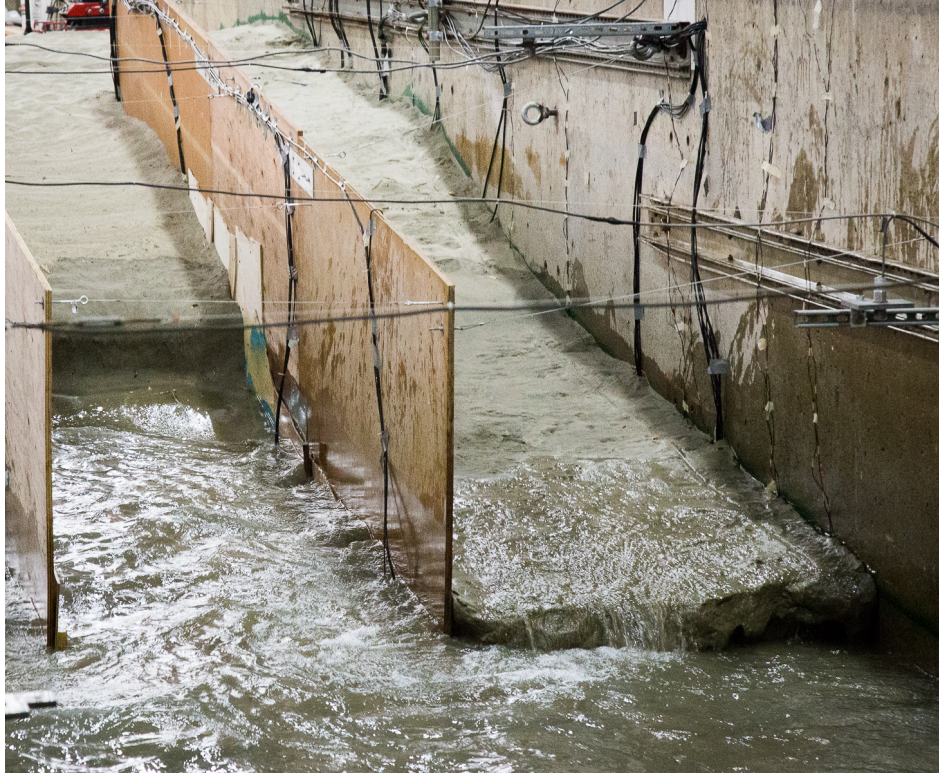
Figure 19. Bio-cemented dune during wave testing in the Large Wave Flume (right) adjacent to the untreated dune experiencing significant erosion (left) (Montoya et al. 2021)
